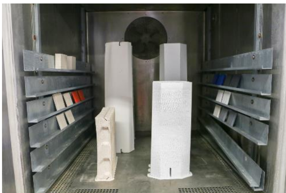
Figure 1: The climatic chamber loaded with samples and prototypes in LPM Lab
